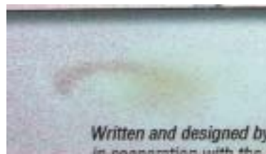
Discoloration from exposure to 30 seconds of open flame
